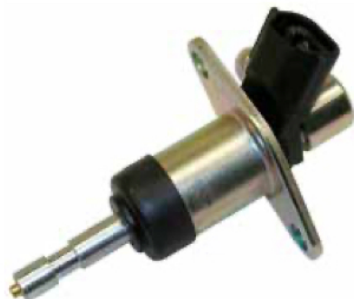
Injector LPG used on Mazda engines REF 136TA3200
